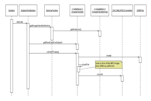
Figure 6.1: SRB-JARGON based image data retrieval and on-the-fly image conversion sequence diagram.
