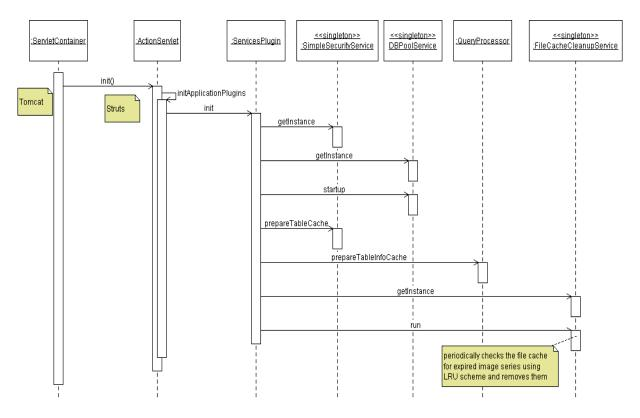
Figure 2.3: Servlet container-Struts initialization sequence diagram.
