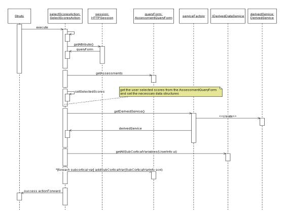
Figure 3.2: Selecting a score Struts action sequence diagram.
