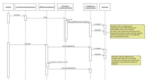
Figure 6.2: SRB Scommand based image series download and AFNI conversion sequence diagram.
