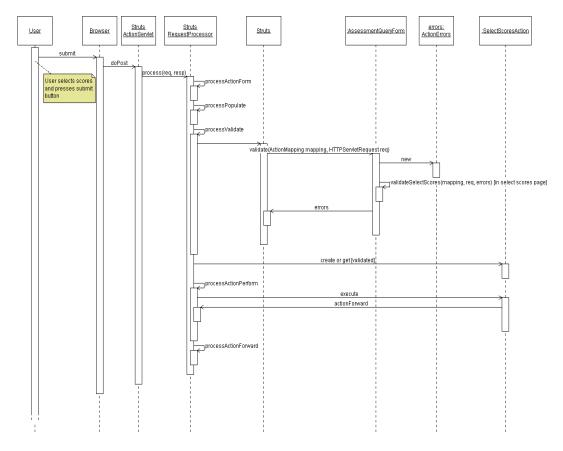
Figure 2.1: User-Struts-Application Interactions for web-tier side form validation and action processing.
