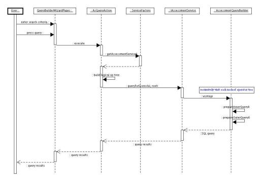
Figure 5.1: High level sequence diagram for assessment query building use case.
