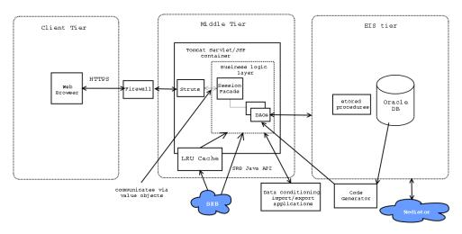
Figure 1.1: High level architecture of UCSD Human Imaging Database User Interface.
